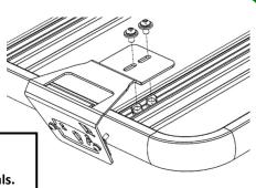
**NOTE-**Ensure the channel nuts are 90 degrees to the channels.
