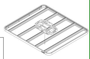
**NOTE-**Ensure the channel nuts are 90 degrees to the channels.
