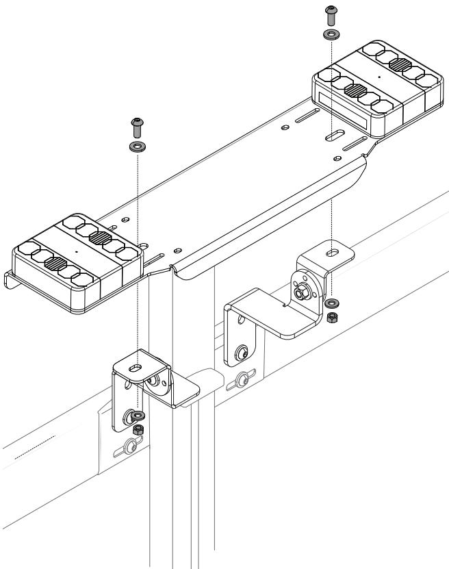
**6** Using the M5 screws and flange nuts provided, attach the license plate.
