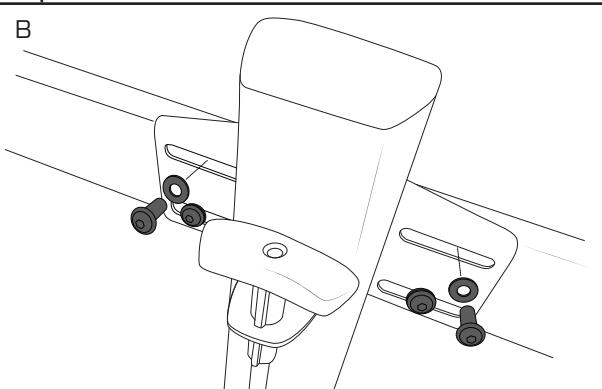
**2** Position wheel tray so its threads are centred withing the corresponding slots.
