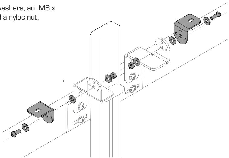
**5** Position LED light board over brackets and fit with M8x20mm dome head screws, 2x flat washers and a nyloc nut.
