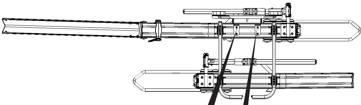
A) Install 4x turn channel nuts into the c-channel of the Gigawatt carrier.
