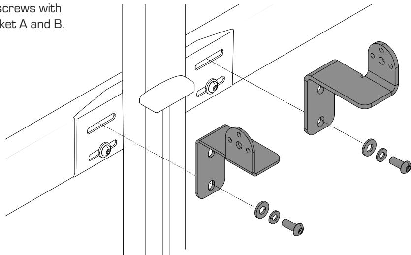
**NOTE** For installation to the Rockymounts Gigawatt, M6 hardware is used.
